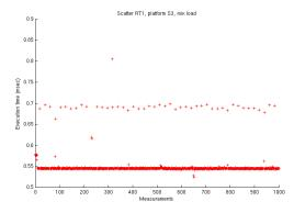
Difference between a run with interrupts disabled and another with SCHED\_FIFO priority on a CPU that does not handle interrupt, except the local timer interrupt (tick)
