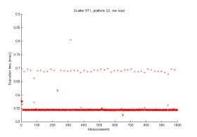
Difference between a run with interrupts disabled and another with SCHED\_FIFO priority on a CPU that does not handle interrupt, except the local timer interrupt (tick)
